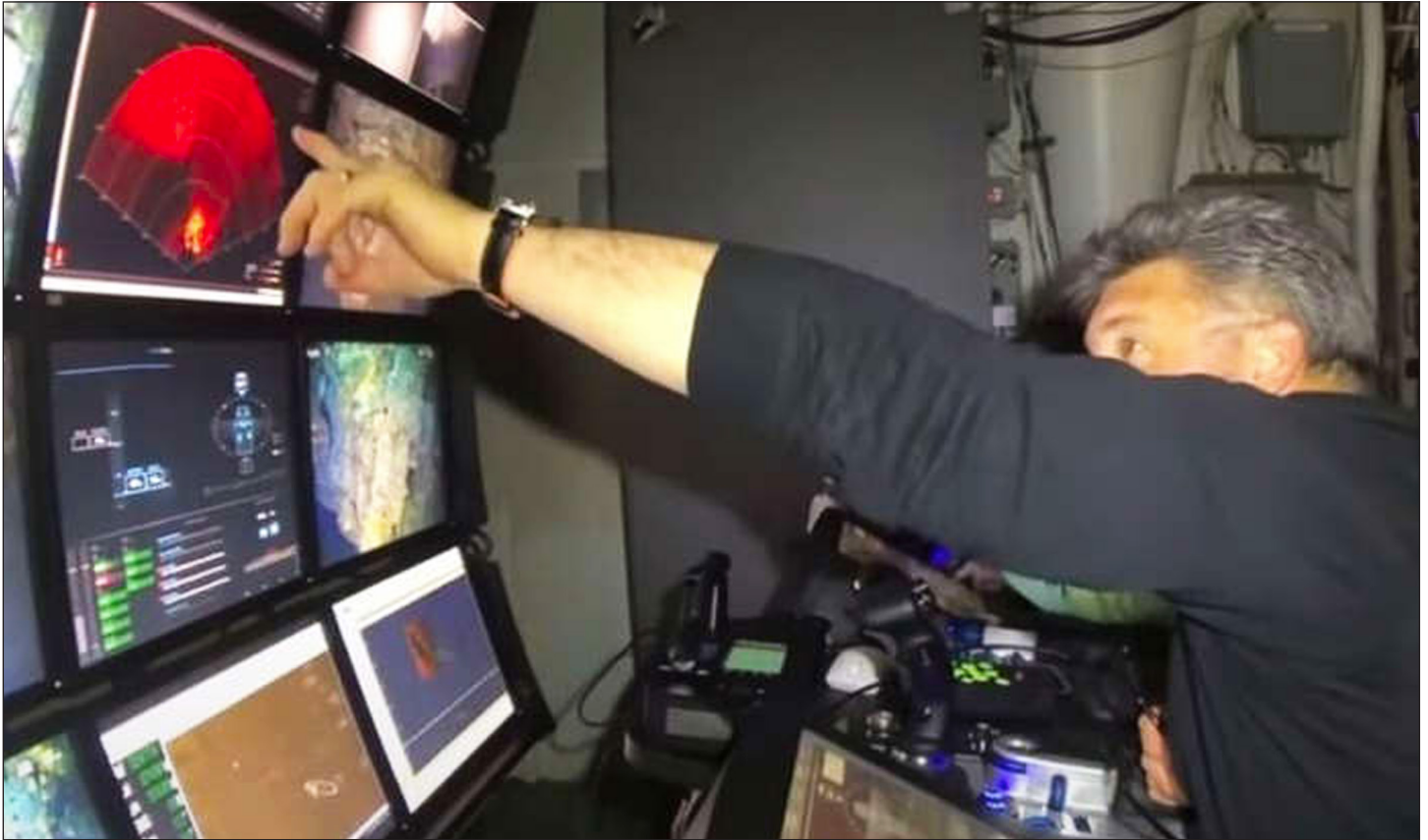
Team leader Tim Taylor uses sidescan sonar to search the bottom for lost subs—including Stickleback .
